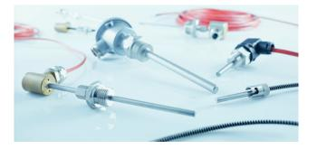
screw-in housing and EM24 / EM38 head made of brass. aluminum or stainless steel. DIN connector head Type A / B / BUS / BUZ / MA, bayonet lock. industrial connector -60°C +400°C / -94°F +752°F 100 Ω at 0°C 2-, 3- or 4-wire circuit or plug connector recommended 0.3 ... 1.0 mA max. 25 mA from 0.5 kV / AC 50 Hz / 1 min., shrinking tube on request e.a. single itzes, hose line AWG28 to AW20 according to customers specification dust- and waterproof versions (IP66)
