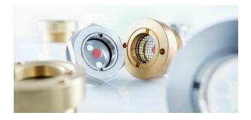
version: inspection glass -40°C ... +105°C / -40°F ... +221°F temperature range: potection system: two-chamber system with a stainless-steel protective grid collision: special outer glass pane resistant to impact of objects up to m = 30g / v = 50 m/sthread: G1", G1¼", G1½", G2", M48x1,5, M42x1,5, M60x2 (other threads on request) IP66 / IP68 protection: housing: brass, aluminum or stainless steel protective grid: stainless steel special design: on request DIN FN 61373 cat. 3 coonformity:
