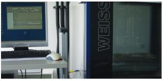
Test bed for the generation of environmental influences, such as temperature and humidity, under laboratory conditions.
