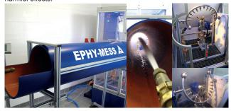
IP X5 test, "Protected against water jets" Protection against ingress of water jets (12,5 l/min.). Water, which is pointed from any direction in jets at the enclosure shall have no harmful effects.
